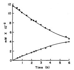
The reaction of p-nitronitrosobenzene (1b) with glyoxylic acid as a function of time. The reaction was initiated by the addition of sufficient 1b as a concentrated solution in ethanol to give an initial concentration of 0.117 mM in a 5.0 mM solution of glyoxylic acid in pH 6.0, 0.05 M, KH<sub>2</sub>PO<sub>4</sub> buffer at 25 °C. The concentrations of reactant 1b ( $\bullet$ ) and product 2b ( $\bigcirc$ ) were determined by direct HPLC analysis at the indicated sampling times.
